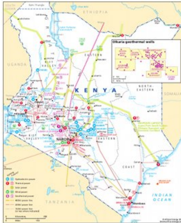
Figure 26 - Planned transmission grid (yellow lines) & geothermal resources (pink circles) (African Energy, 2012)
